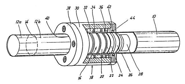
Inside the cylinder, the piston is driven by a pressurized fluid. Stoll patent, col. 3, Il. 13-19. As the piston travels through the cylinder, the magnetically coupled sleeve follows the piston along the outside of the cylinder. <u>Id.</u>
